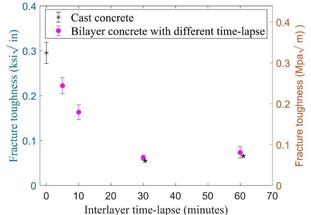
\* Approximate fracture toughness as these specimens were not linearly elastic
