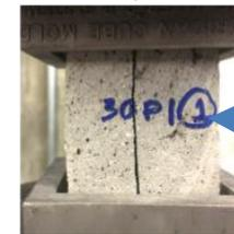
Layers separate before the specimen fail
