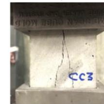
c) Bilayer specimen with loading perpendicular to the interlayer surface
