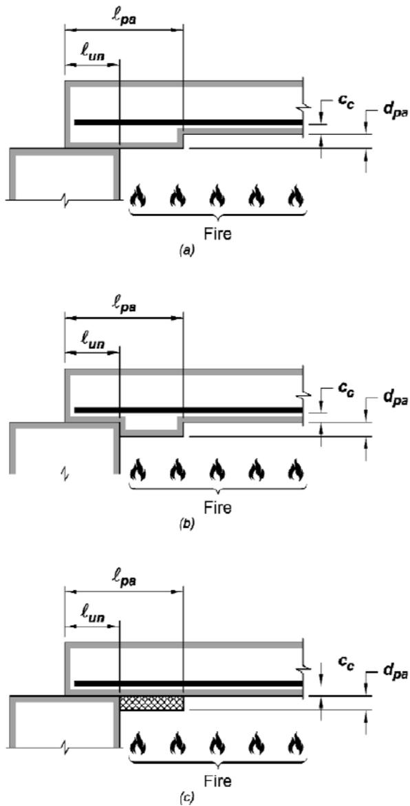
Fig R7.2.4a-c—Protection of GFRP reinforcement near supports.
