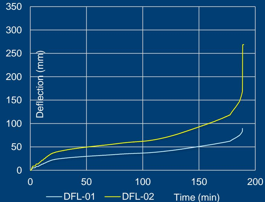
Both slabs sustained load equal to 45% of ultimate capacity for more than 180 minutes.
