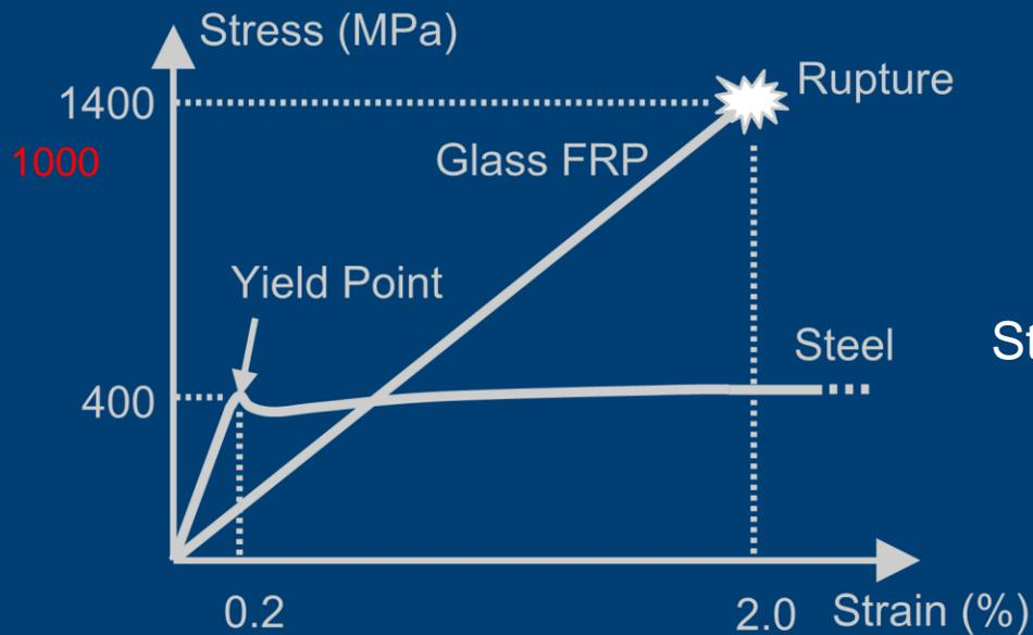
Stress strain curves for GFRP and steel reinforcement (ISIS 2006)
