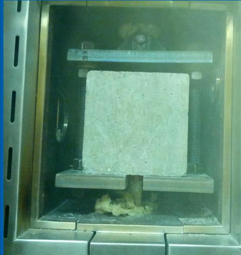
Pullout sample placed in furnace
