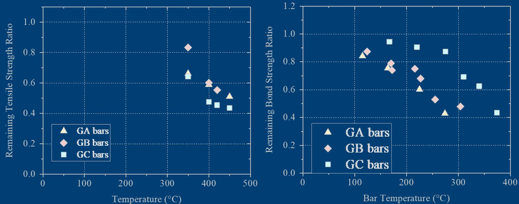
Fig. 1 Remaining residual properties of GFRP bars: (a) tensile strength; (b) bond strength
