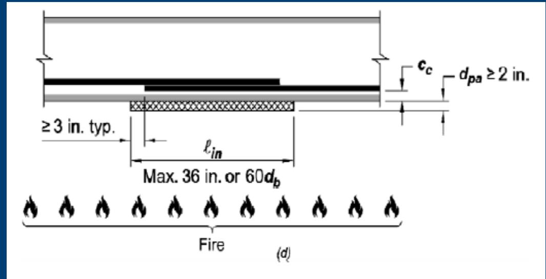
Fig R7.2.4.d—Insulation at spliced GFRP reinforcement.
