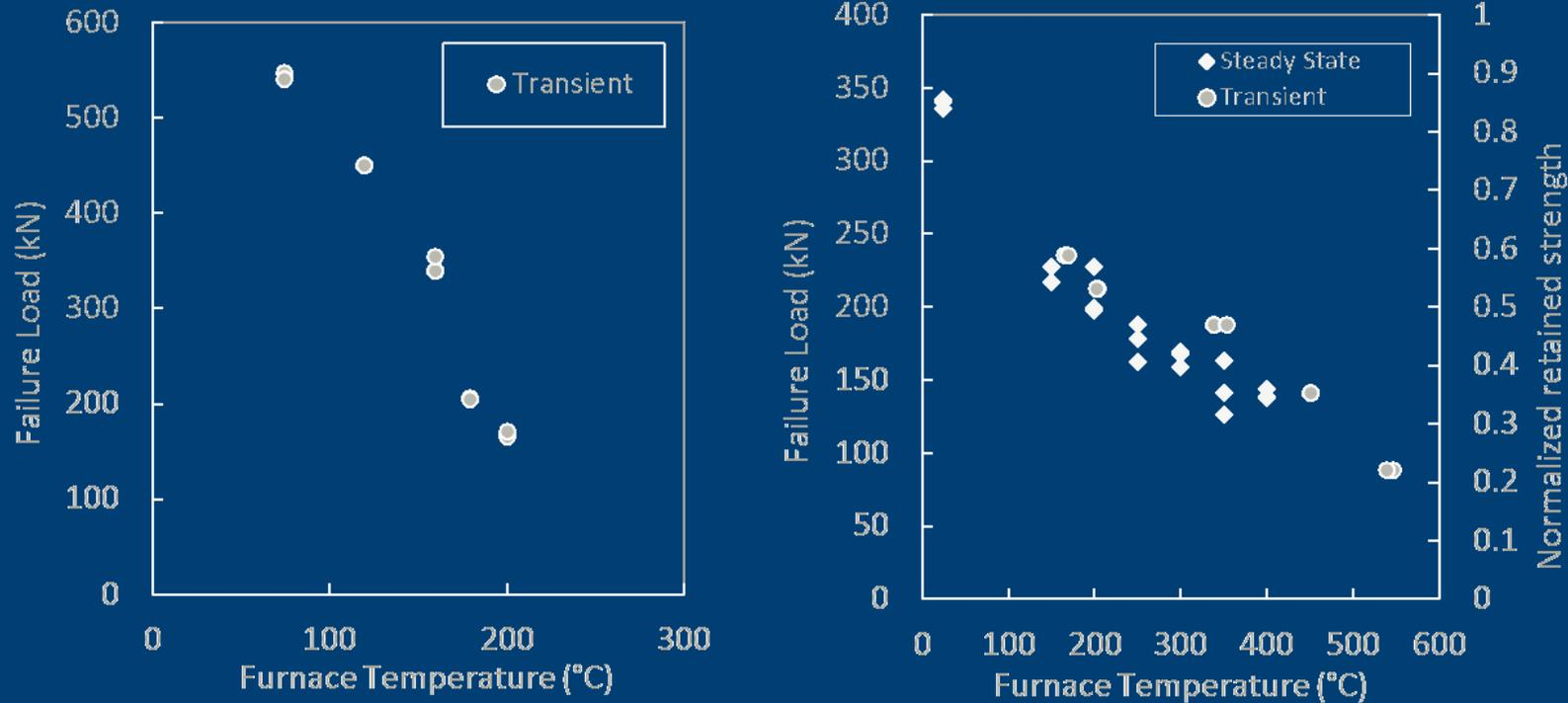
(Left) Tensile strength degradation in Transient tests (#5 GFRP bars);
