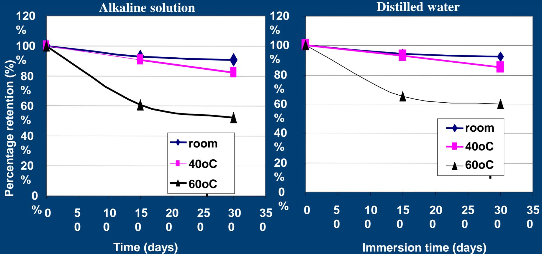
Two competing mechanisms: post-cure and degradation.
