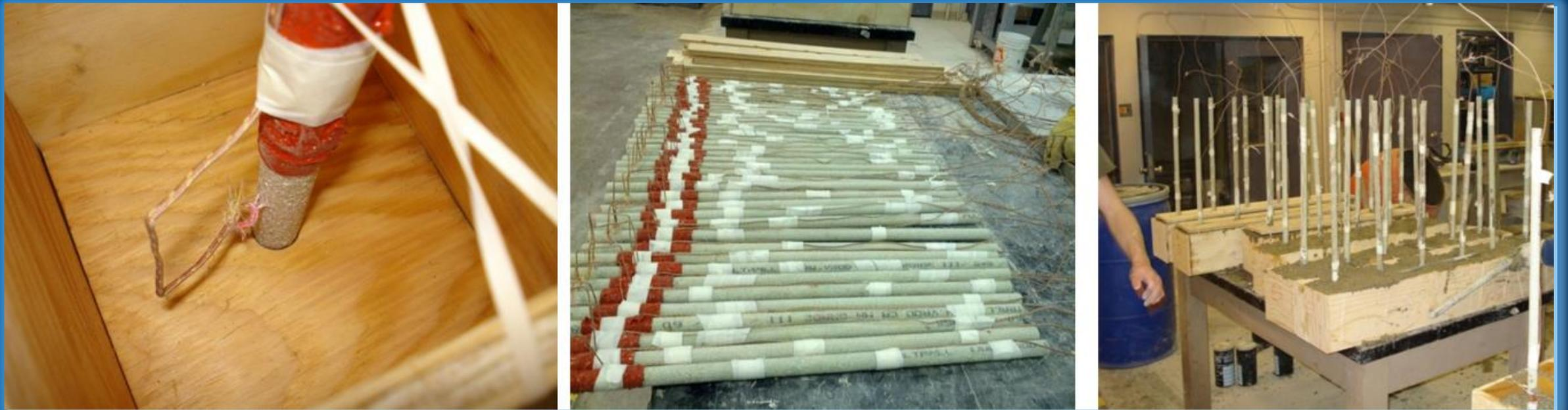
Thermocouple placements (Right); bond breaker (Middle); concrete casting (Left)
