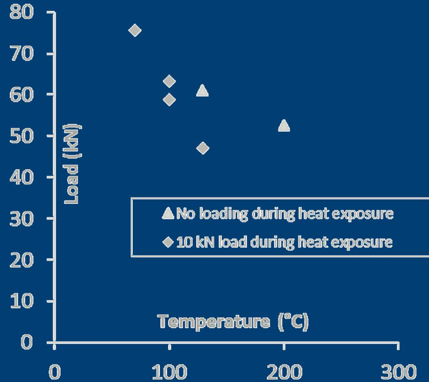
Residual strength (after fire) pullout test results
