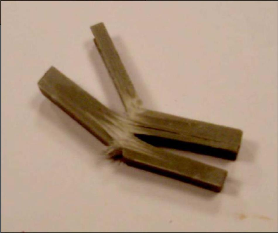
Fig. 2: Fractured CVN specimen after the test
