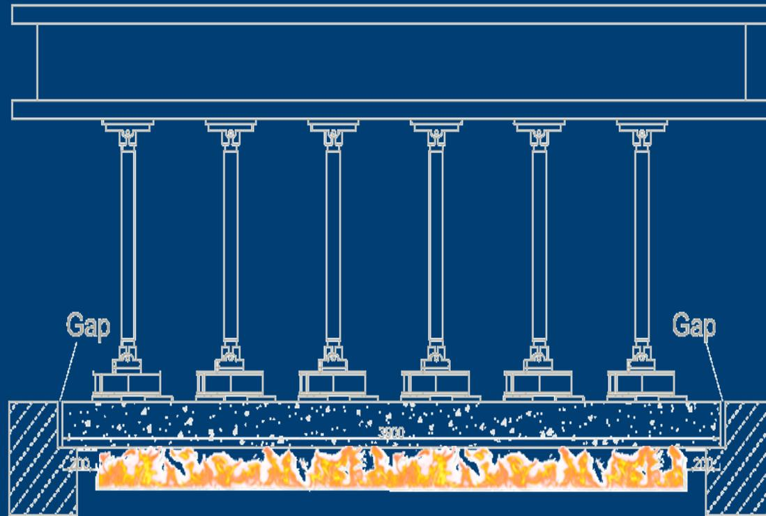
Test Setup at NRC— slab 1200 x 3900 x 200mm thick
