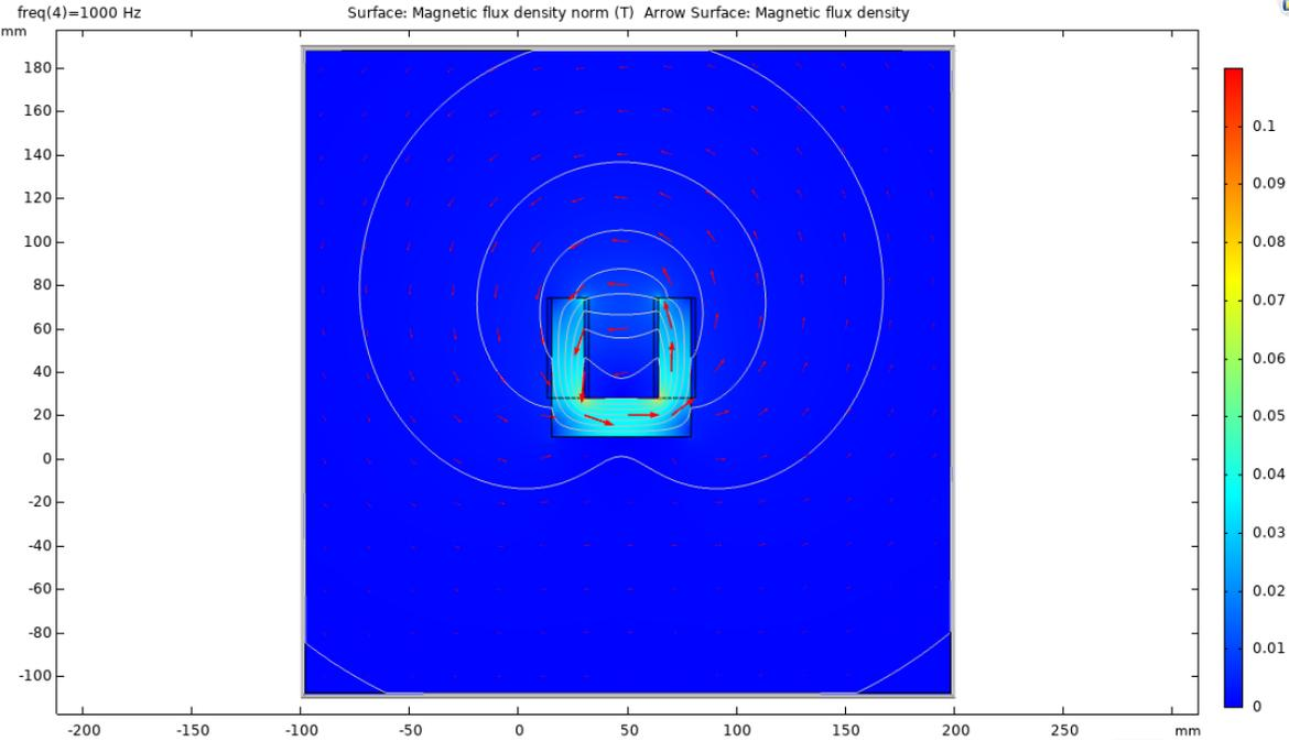
Left: large cross-sectional area (100 x 80mm) magnet with similar (75x75) field pattern with a smaller one.
