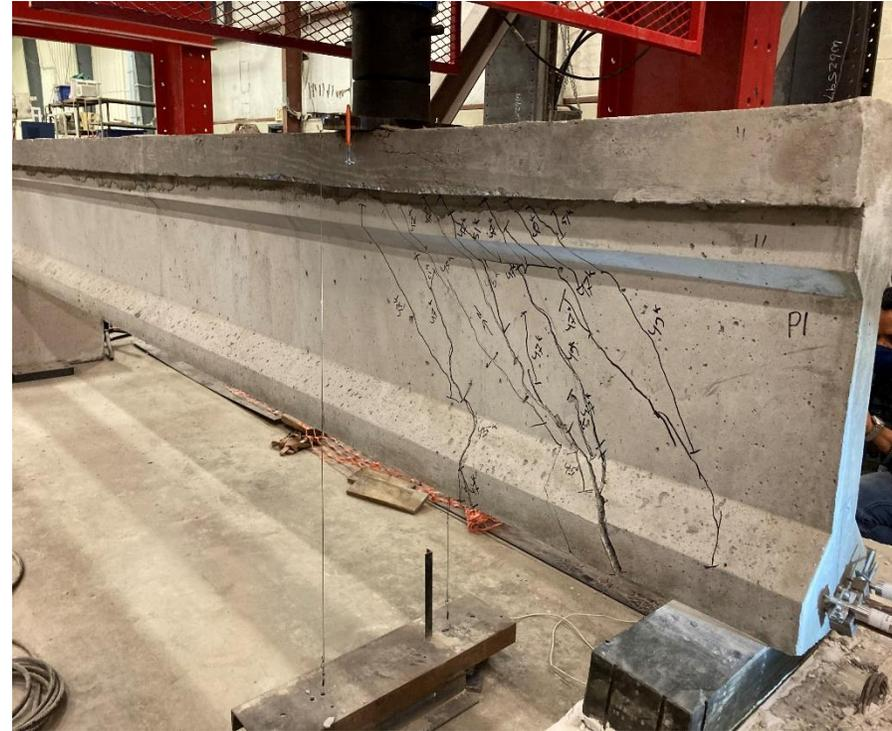
Prestressed beam with bond-shear cracks
