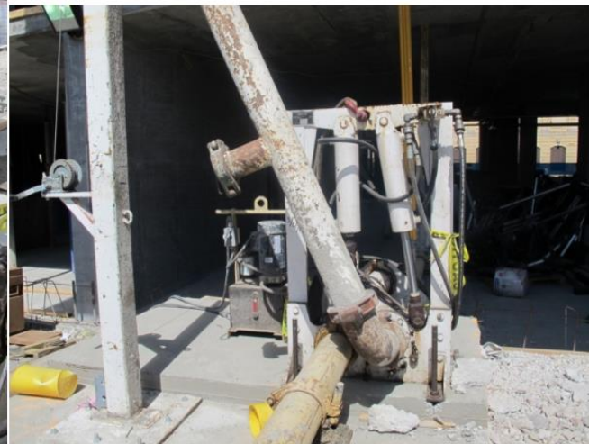
This discharge pipe sends the concrete back into the truck to be taken away. Notice the trap basket to catch the sponge ball
