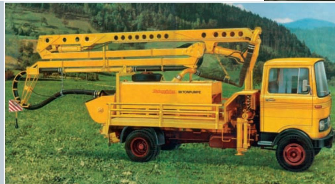
First Putzmeister truck-mounted concrete pump with M 16 boom and 100 mm delivery line on Mercedes-Benz L 808
