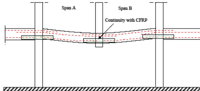
*Figure 1.2 Behavior of Rehabilitated Structure after Removal of the Column*
