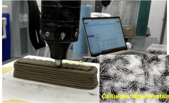
3D printed "alkali-activated- cellulose nanomaterial" composites
