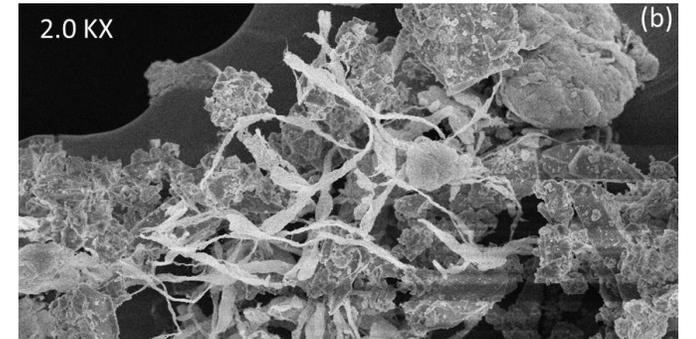
SEM image of CNTs deposited on Cement
