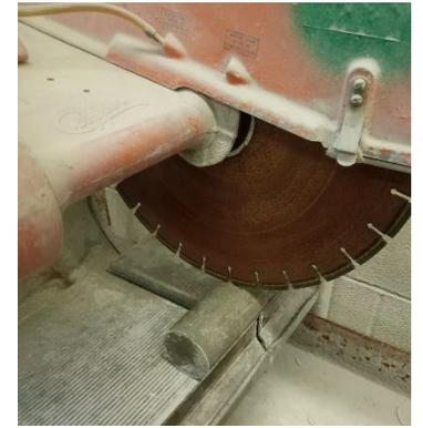
Saw-cutting specimen to 4.5"
