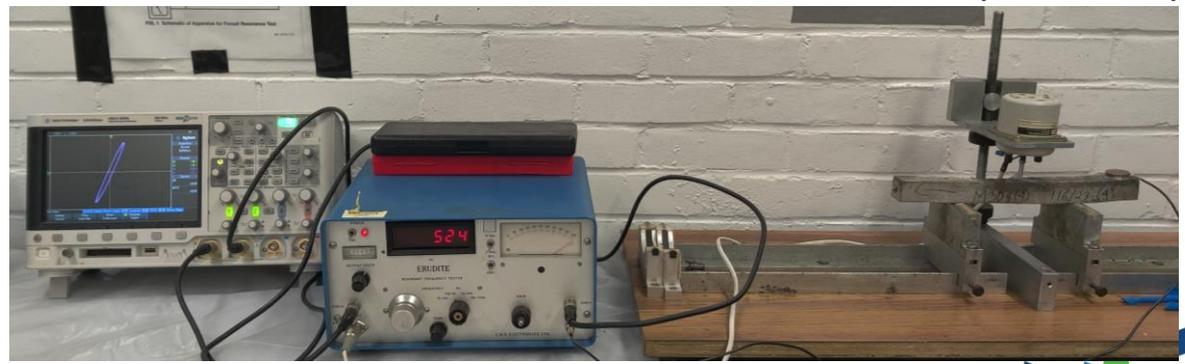
Dynamic Elastic Modulus Resonance Frequency Test (ASTM C215)
