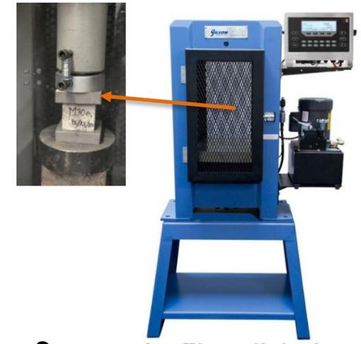
Compressive Strength test (ASTM C 109)
