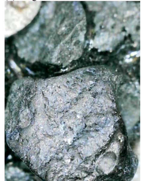
(b) Slag after 120 min of MD Abrasion
