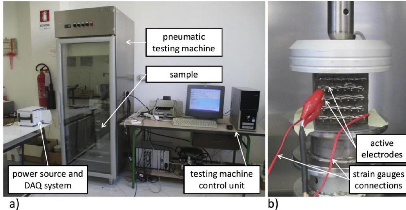
**Fig. 5.** a) Test set-up for strain sensing assessment of the composite materials; b) detailed view of coaxial cables connected to the net electrodes of the sample.
