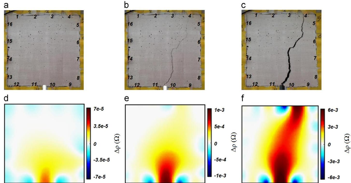
Fig. 7. (a)-(c) Photograph of the sensing skin at three different load levels shown in Fig. 6b, (d)-(f) ERT images of sensing skins at three different load levels shown in
