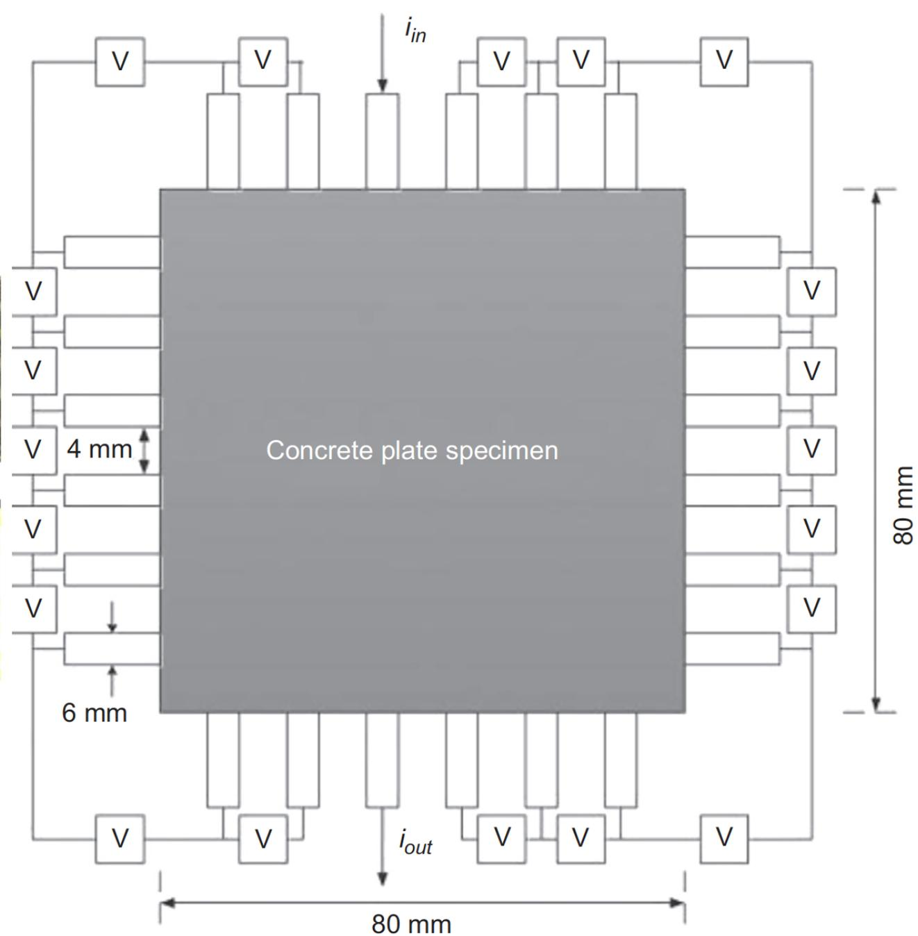
**figure 11.4** Schematic of an EIT system (Gupta et al., 2016).
