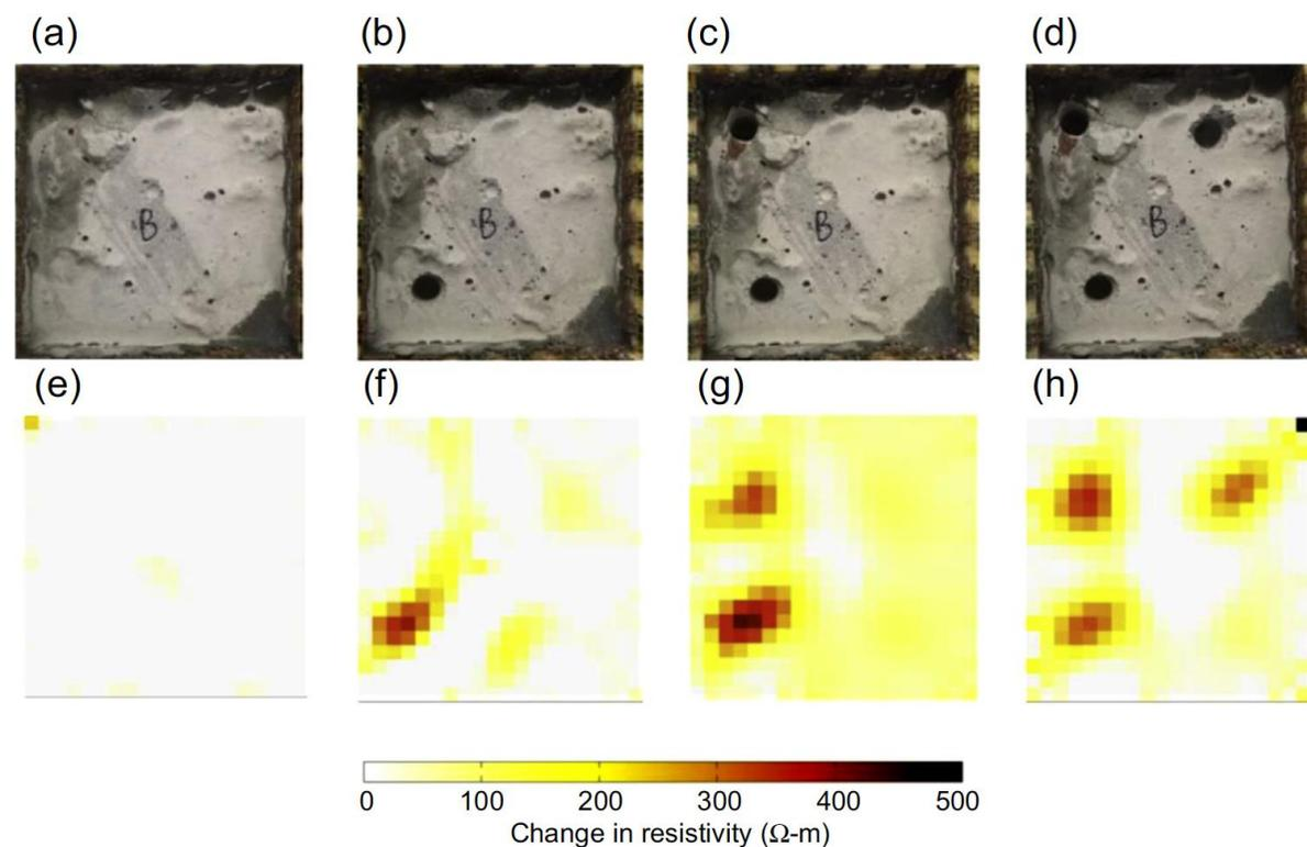
**Figure 11.5** Damage detection tests were performed on the concrete plates cast using large aggregates coated with MWCNT-latex thin films (Gupta et al., 2016).
