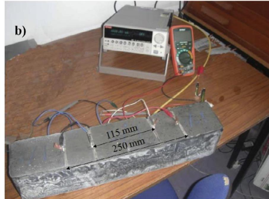
**Fig. 4.** Experimental setup. (a) Mechanical and piezoresistive characterization and (b) electrical characterization.
