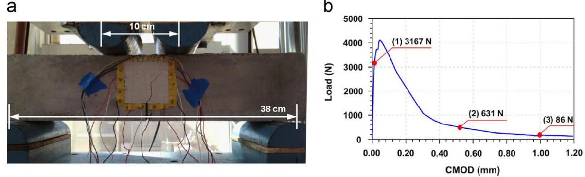
Fig. 6. (a) Photograph of the notched beam, (b) load versus Crack Mouth Opening Displacement (CMOD) curve of the notched beam.
