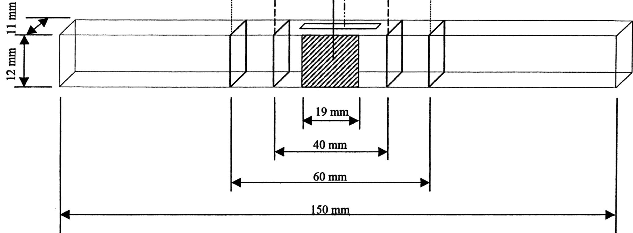
Fig. 1. Sample configuration for measuring the transverse electrical resistivity during uniaxial compression.
