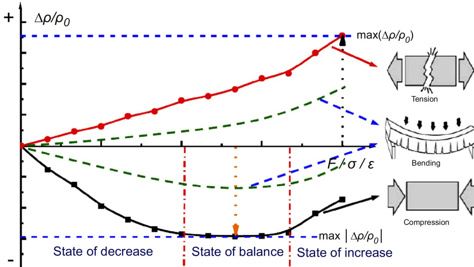
Figure 11.8 Typical sensing behavior of ISSC under loading (Han et al., 2015d).
