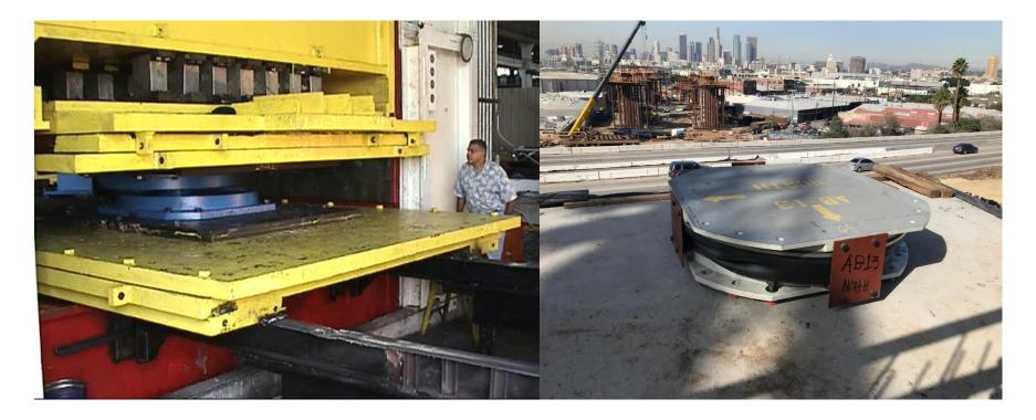
First bridge in the world to use next-generation triple-pendulum friction-bearing technology, developed for this project to stiffen at a predetermined displacement
