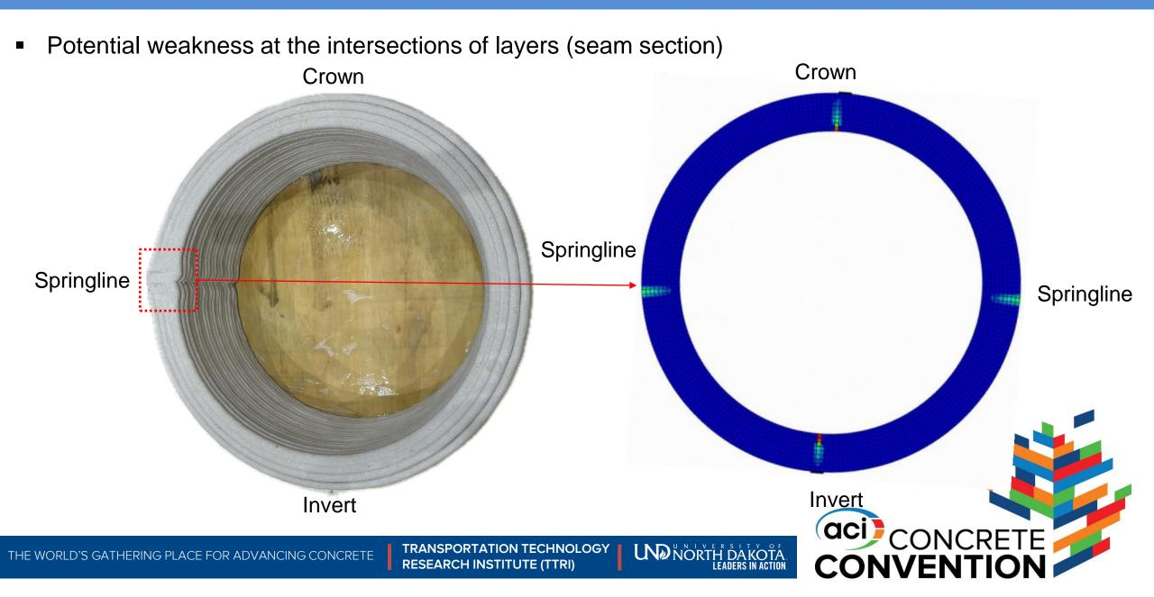
Crack propagation and failure behavior
