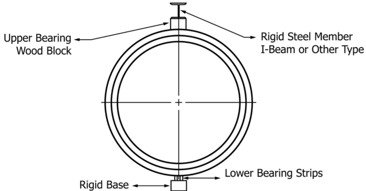
Three-Edge-Bearing Test, Circular Pipe
