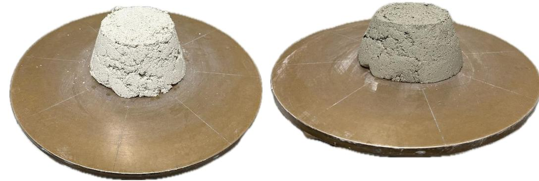
Demolded samples for flow table test at 50 minutes
