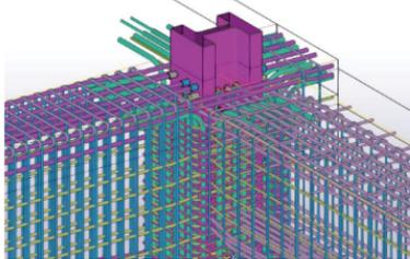
Once the reinforcing steel is modeled in 3D, clashes or interference from structural steel members become very obvious.
