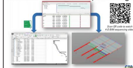
A four dimensional BIM model contains additional dimensional information, known as a scheduling data or the time element. Therefore, 4D BIM is essentially 3D BIM + scheduling/sequencing.
