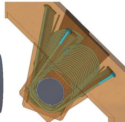
3D Modeled bars for complex shapes as shown above, make it easier for the fabricator to visualize what they bending.
