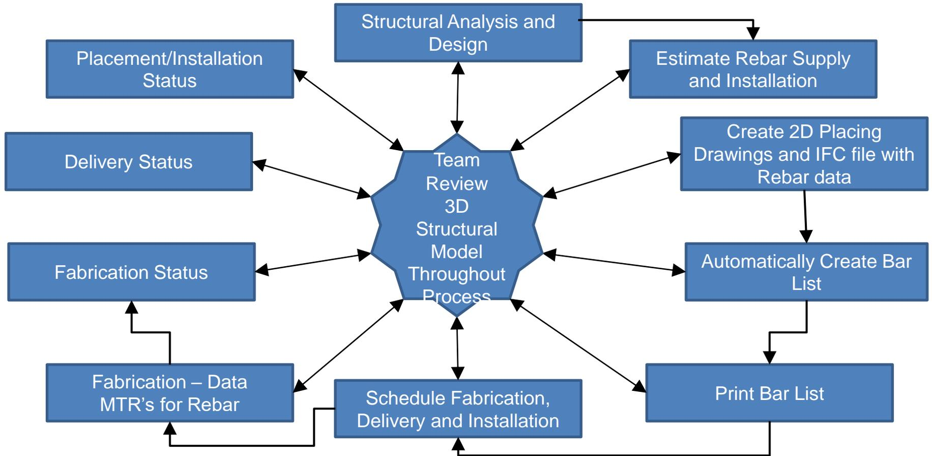
...A truly collaborative rebar workflow utilizing 3D structural model
