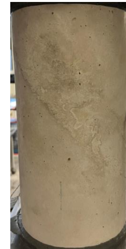
Strut Crossing Cold Joint in Retrofitted Pier Cap (Bayrak, 2020)
