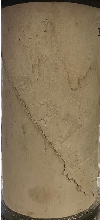
Slant shear failure
