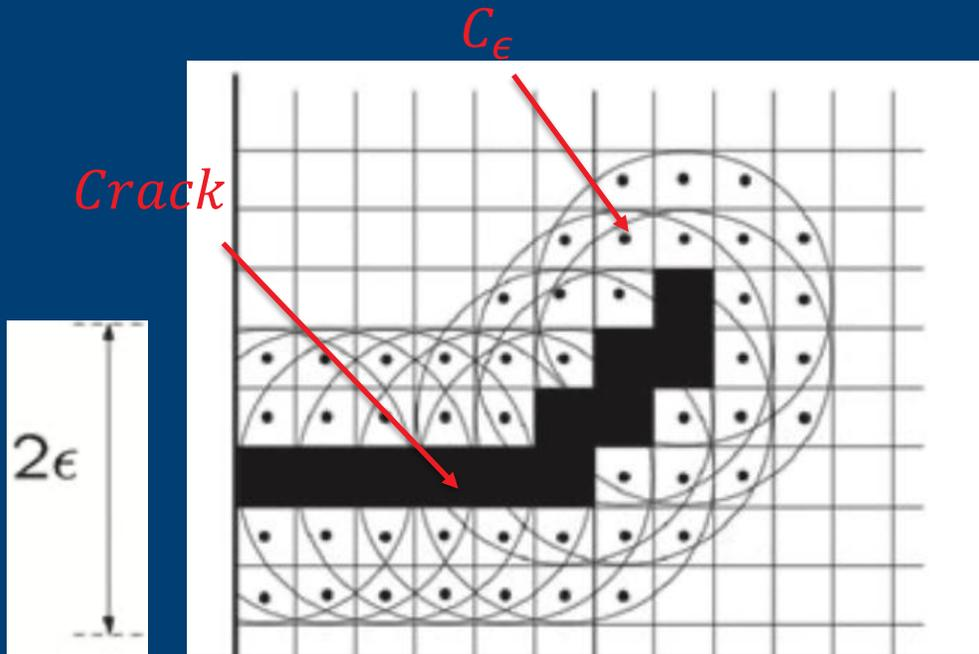
Figure: Square mesh with existing crack
