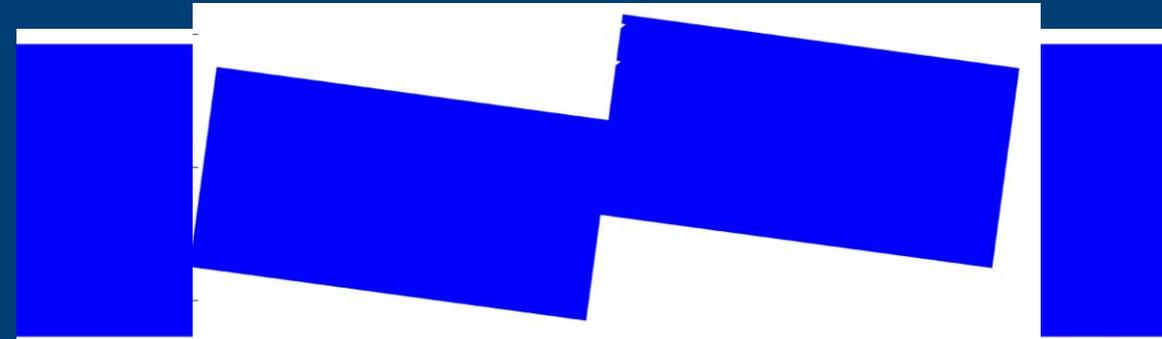
Figure: Mode II fracture
