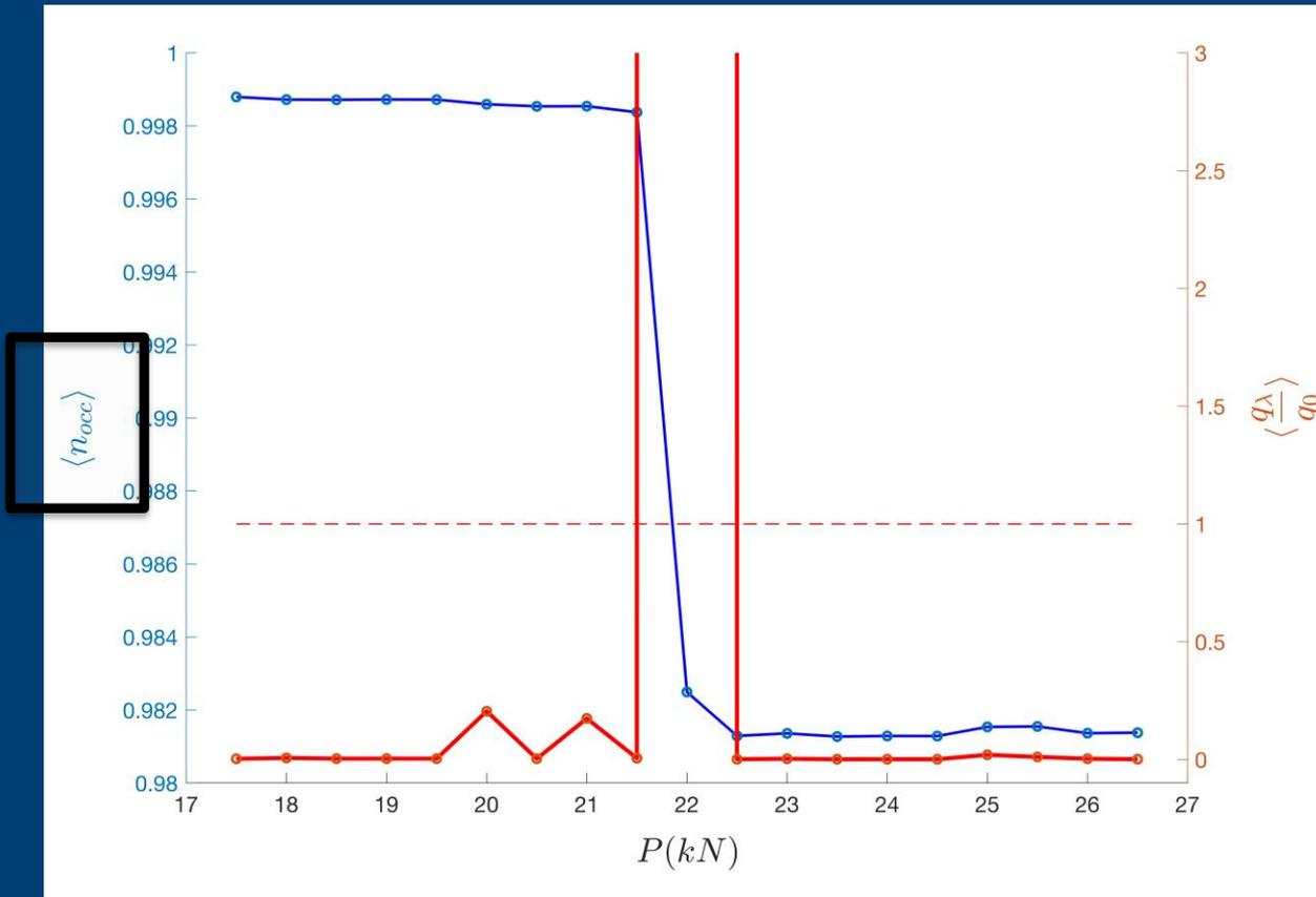
Figure: Critical load detection ( $\frac{a_0}{H} = 0.2$ )
