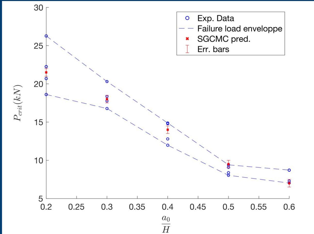
Figure: Fracture load predictions [2]
