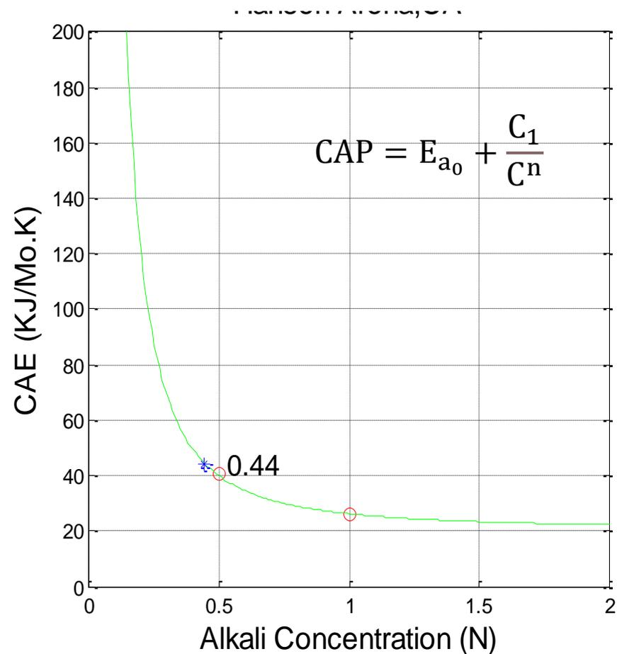
THA is calculated mathematically from the CAP vs alkalinity plot when the slope of Eq. (1) equals -100
