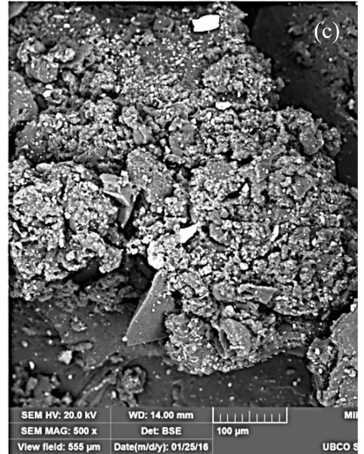
Crumb rubber particles at magnification levels of (a) 28x, (b) 80x, and (c) 500x using Scanning Electron Microscope (SEM)
