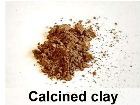
Burned at much lower temperature than clinker and small process emissions
