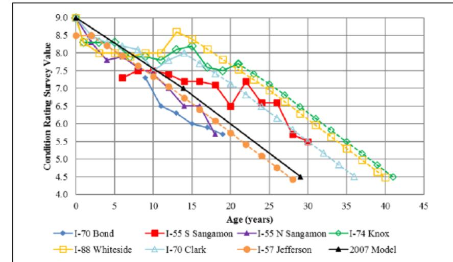
Figure 2. Unbonded concrete overlays condition rating survey values vs. age.
