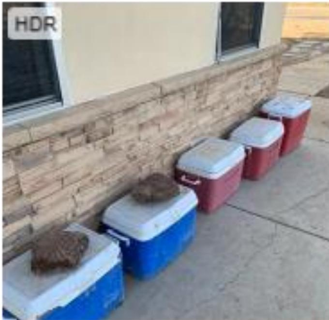
**The blue containers had weight on the lid to seal the cooler + Heat of hydration**
