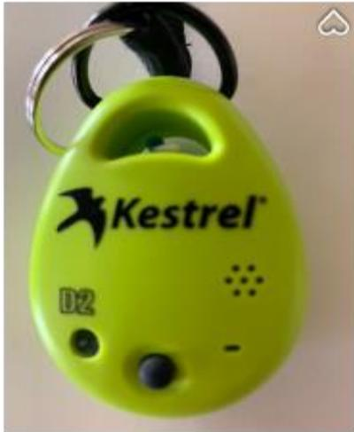
This is a method of getting the temperature, & Relative Humidity of the curing box with the Iphone. Put this on top of the cylinder . Kestrel was at a recent ACI convention.
