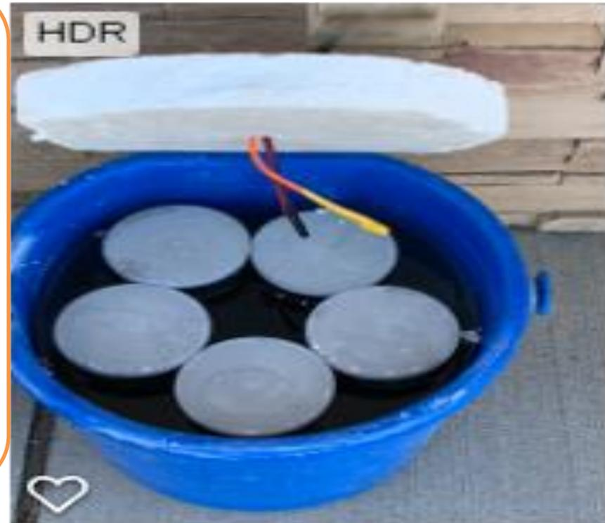
New buckets turn on at 35F and off at 45F air temp.
