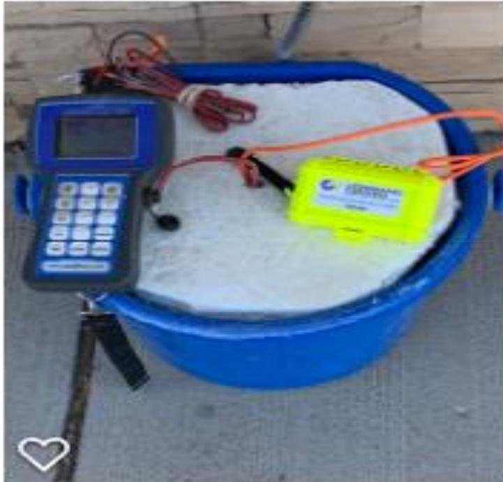
Command center and intellirock sensors use to record temperatures
