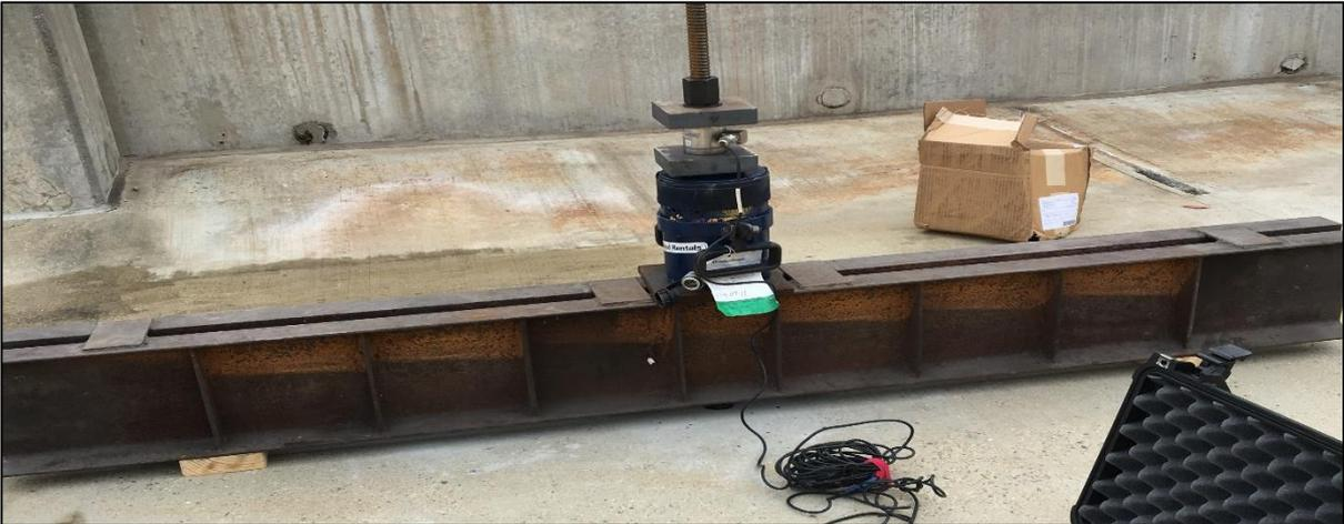
Steel Spreader Beam with High Strength Williams Bar
