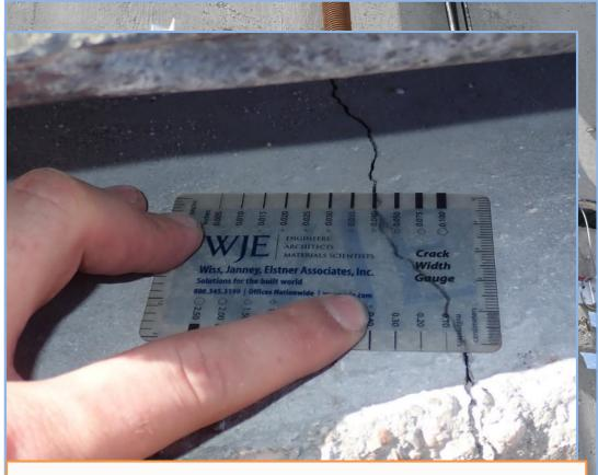
Residual Strain (external): 1,000 με 0.04'' crack / 38'' gage = 1,052 με
