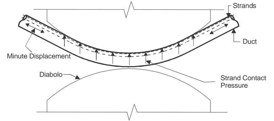
STEP 1: Test set-up
