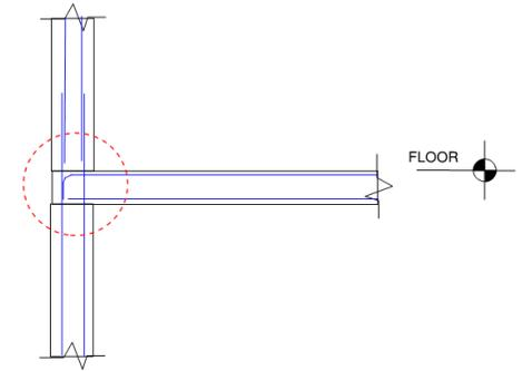
TYPICAL WALL-TO-SLAB CONNECTION DETAIL
