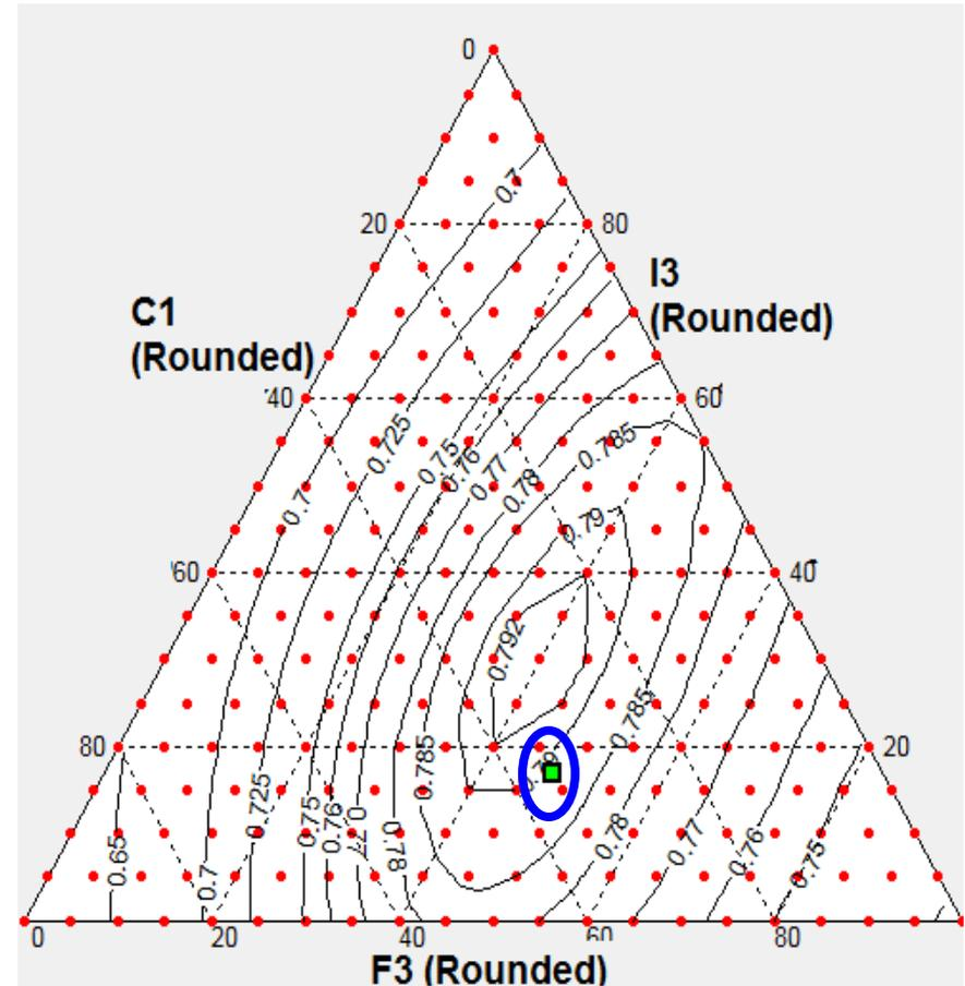
Optimum proportioning of **F**ine, **I**ntermediate, and **C**oarse aggregates increases PD from 0.65 to 0.82
