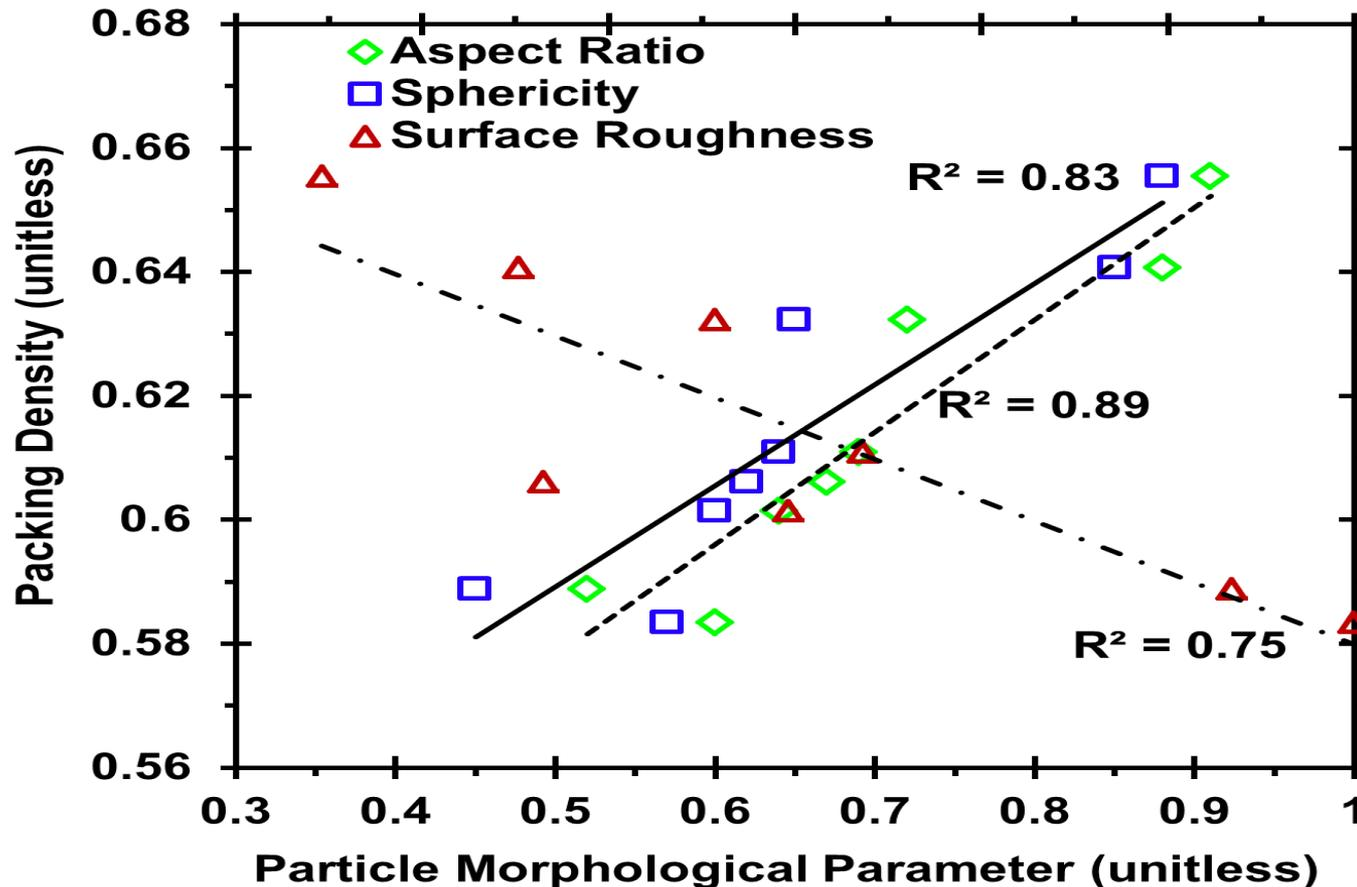
PD is improved with increased aspect ratio and sphericity and decrease in surface roughness
