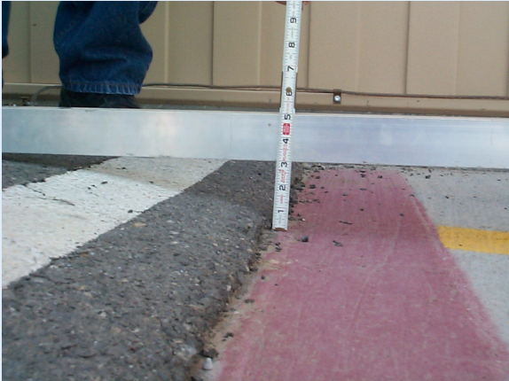
Pavement on left with recycled base, on right without
