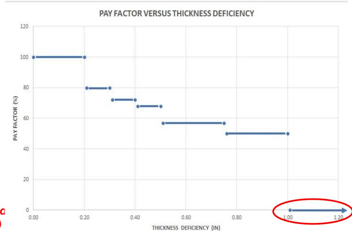
**Concrete Pavement Paid Based on Strength and Thickness**
