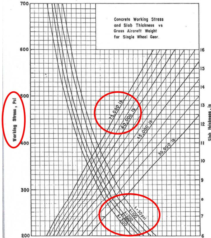
FIGURE 3-10. DESIGN CURVES - RIGID PAVEMENT - SINGLE GEAR
