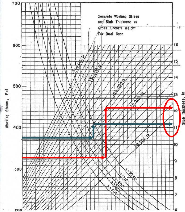
FIGURE 3-11. DESIGN CURVES - RIGID PAVEMENT - DUAL GEAR
