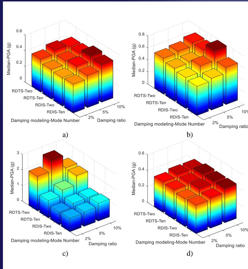
Median fragilities with different frequency ranges for a) System (complete damage state), b) Column (complete damage state), c) Deck unseating at in-span hinge (Extensive damage state, and d) Shear key (moderate damage state)
