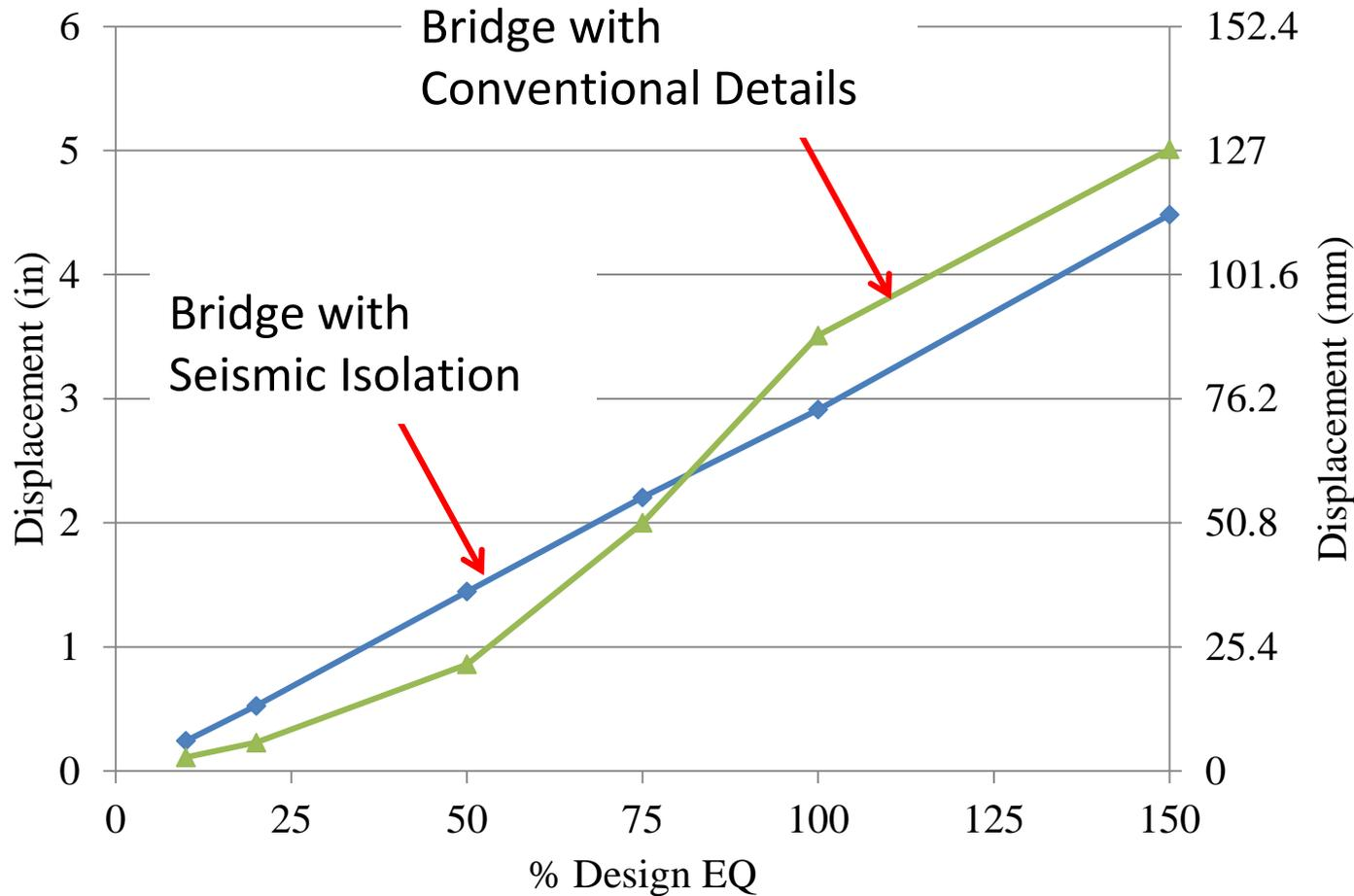
Due to damage in the columns, in addition to effects of in-plane torsional rotation of the curved bridge, the conventional bridge experienced higher displacement at EQ levels beyond the Design EQ.
