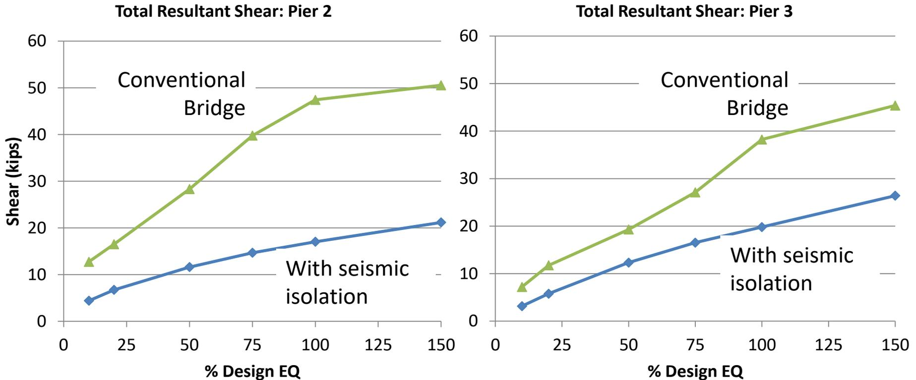
The seismic isolation reduced the column base shear by about 50% at Design EQ level.
