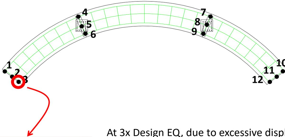
At 3x Design EQ, due to excessive displacements, instability occurred at the isolators at one of the abutments.
