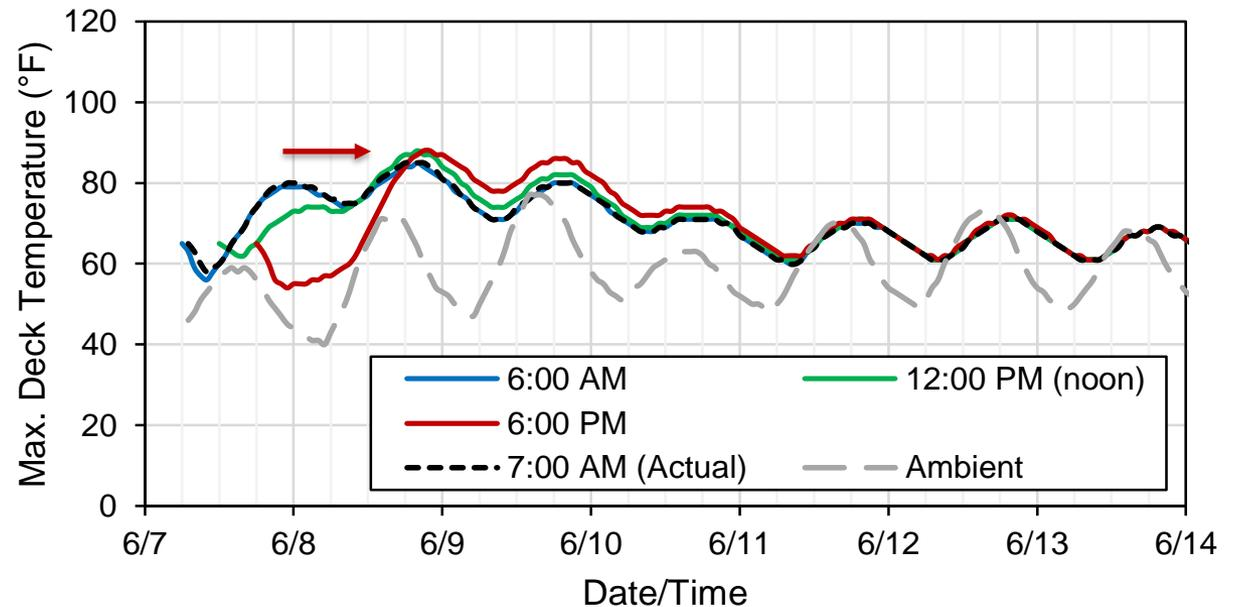
Placing concrete in late afternoon shifts peak temp. difference to Day 2 or 3.
