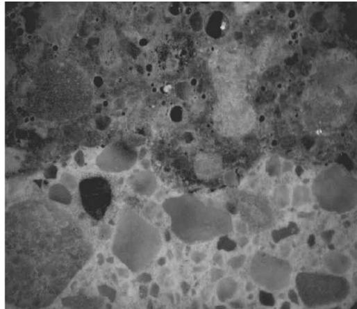
**Figure 3** - Photomicrograph of interface concrete in Core BT-13. It is noted that the repair concrete is well bonded to the existing parent concrete and represents a sound bond. No debris, microcracking or poor consolidation is present. Length of view is approximately 0.35".
