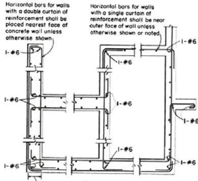
Horizontal bars for walls with a double curtain of reinforcement shall be placed nearest face of concrete wall unless otherwise shown.
