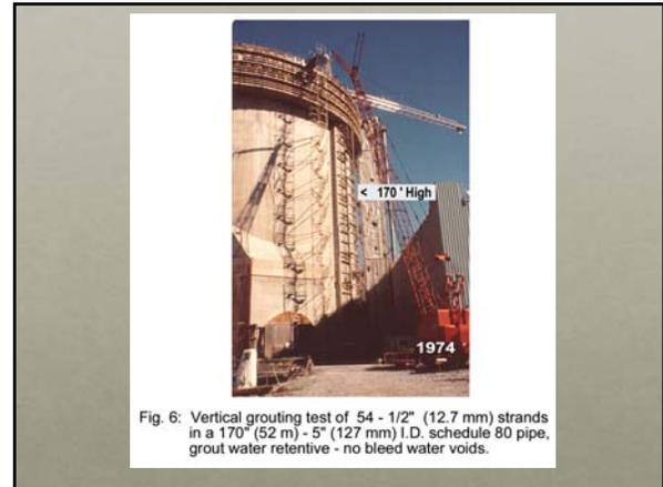
Fig. 6: Vertical grouting test of 54 - 1/2" (12.7 mm) strands in a 170" (52 m) - 5' (127 mm) I.D. schedule 80 pipe, grout water retentive - no bleed water voids.
