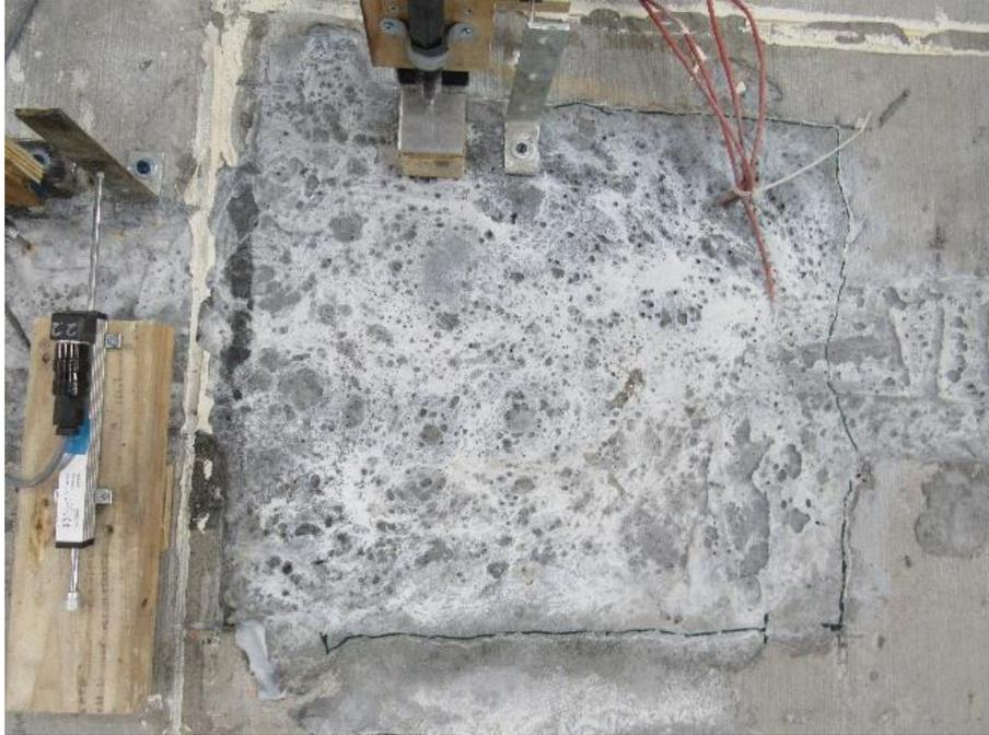
**Minor cracks at the edge of Pocket and Continuous joints at girder failure.**
