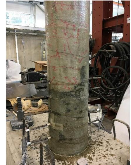
Repaired pier with GFRP confinement
