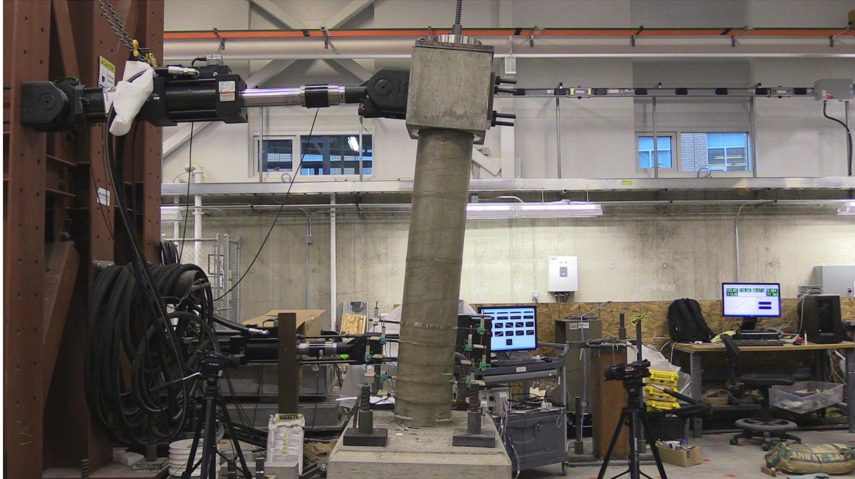
GFRP retrofitted pier under lateral cyclic test
