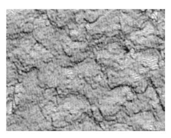
Fig. 1—Typical plus or minus 1/4 in. profile (From ICRI Guideline No. 03732 Profile No. 7). This is standard recommended surface profile for low-pressure spray-applied mortars.
