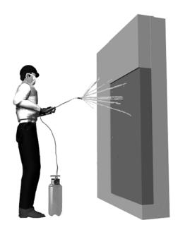
Fig. 6—Application of curing compound.
