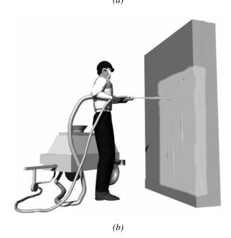
Fig. 4(a) and (b)—Application of mortar with pressure equipment and nozzle.
