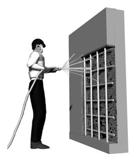
Fig. 3—Presaturate prepared surface with water.
