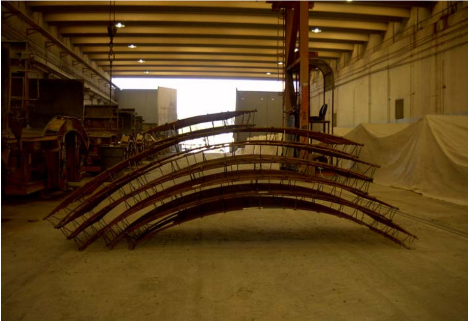
Mercer Street Tunnel Rolled WWR Sheets
