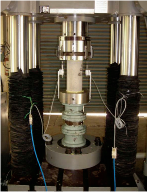
Fig. 2—Modulus of elasticity test setup.
