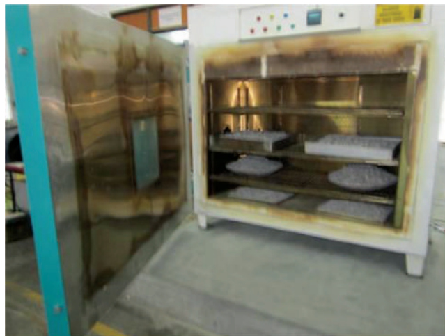
Fig. 1—Oven used for heating recycled concrete aggregate.
