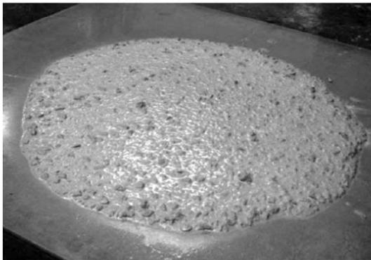
FIG. X1.2 VSI = 1 – Concrete Shows Slight Bleeding Observed as a Sheen on the Surface.
