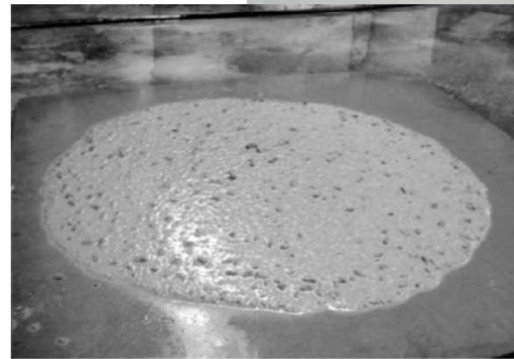
FIG. X1.3 VSI = 2 – Evidence of a Mortar Halo and Water Sheen.
