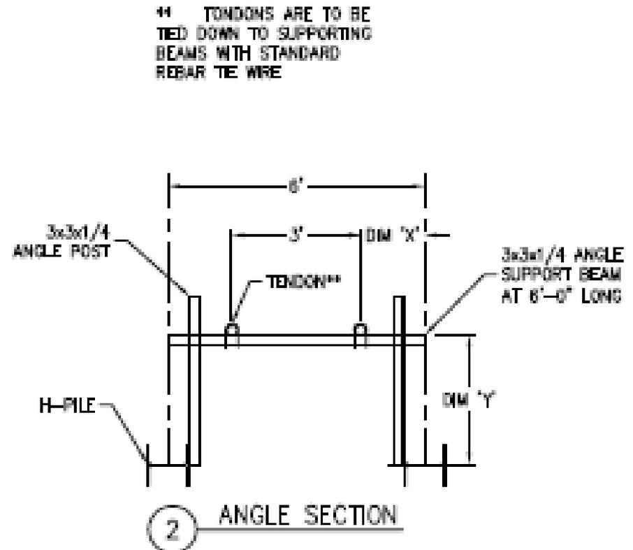
\*\* TENDONS ARE TO BE TIED DOWN TO SUPPORTING BEAMS WITH STANDARD REBAR TIE WIRE
