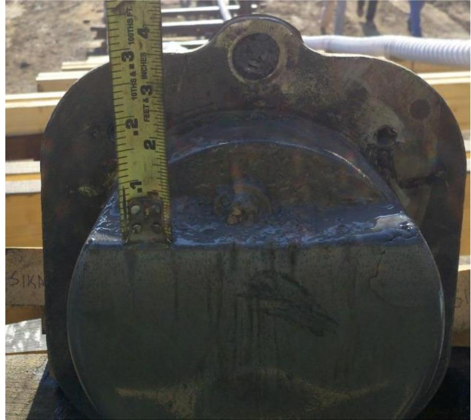
Grout 2 void and soft grout
