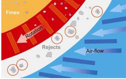
working principle 3<sup>rd</sup> generation separator
