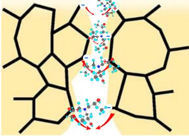
⇒ ensured cracking of particles leads to a faster grinding
