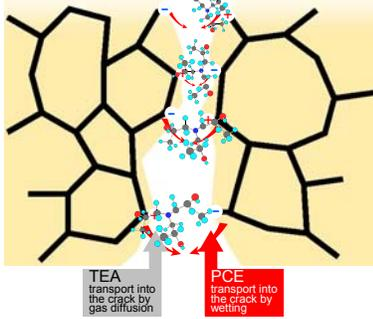
TEA transport into the crack by gas diffusion
