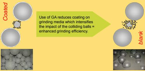
Use of GA reduces coating on grinding media which intensifies the impact of the colliding balls = enhanced grinding efficiency.
