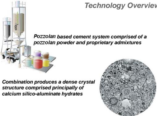
**Pozzolan based cement system comprised of a pozzolan powder and proprietary admixtures**
