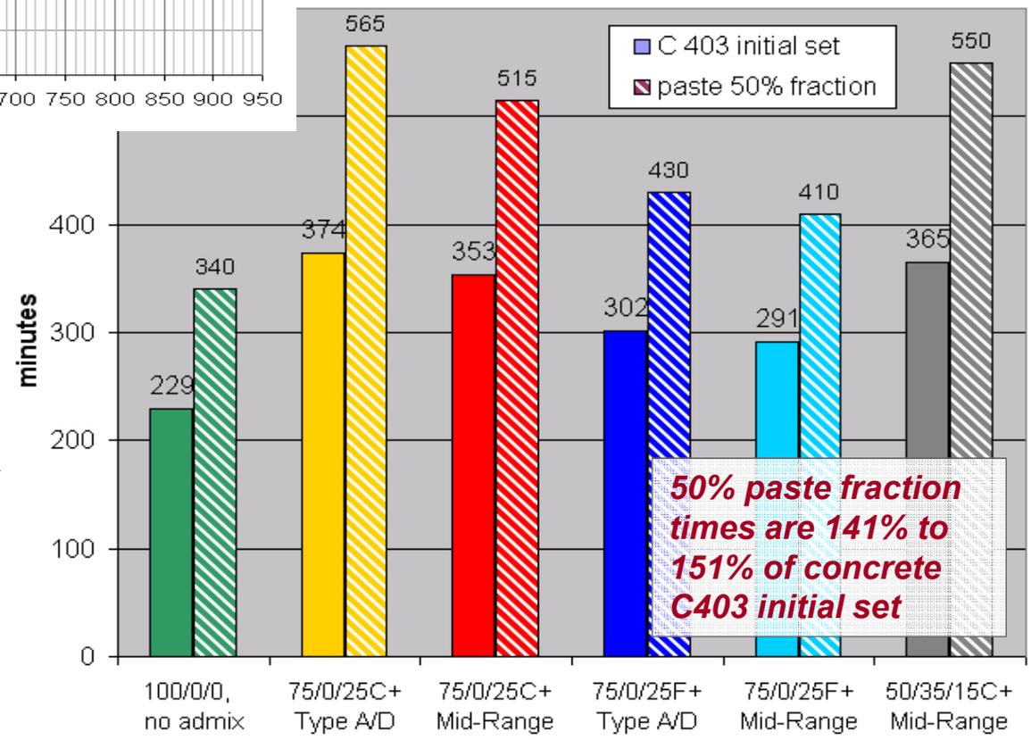
**50% paste fraction times are 141% to 151% of concrete C403 initial set**
