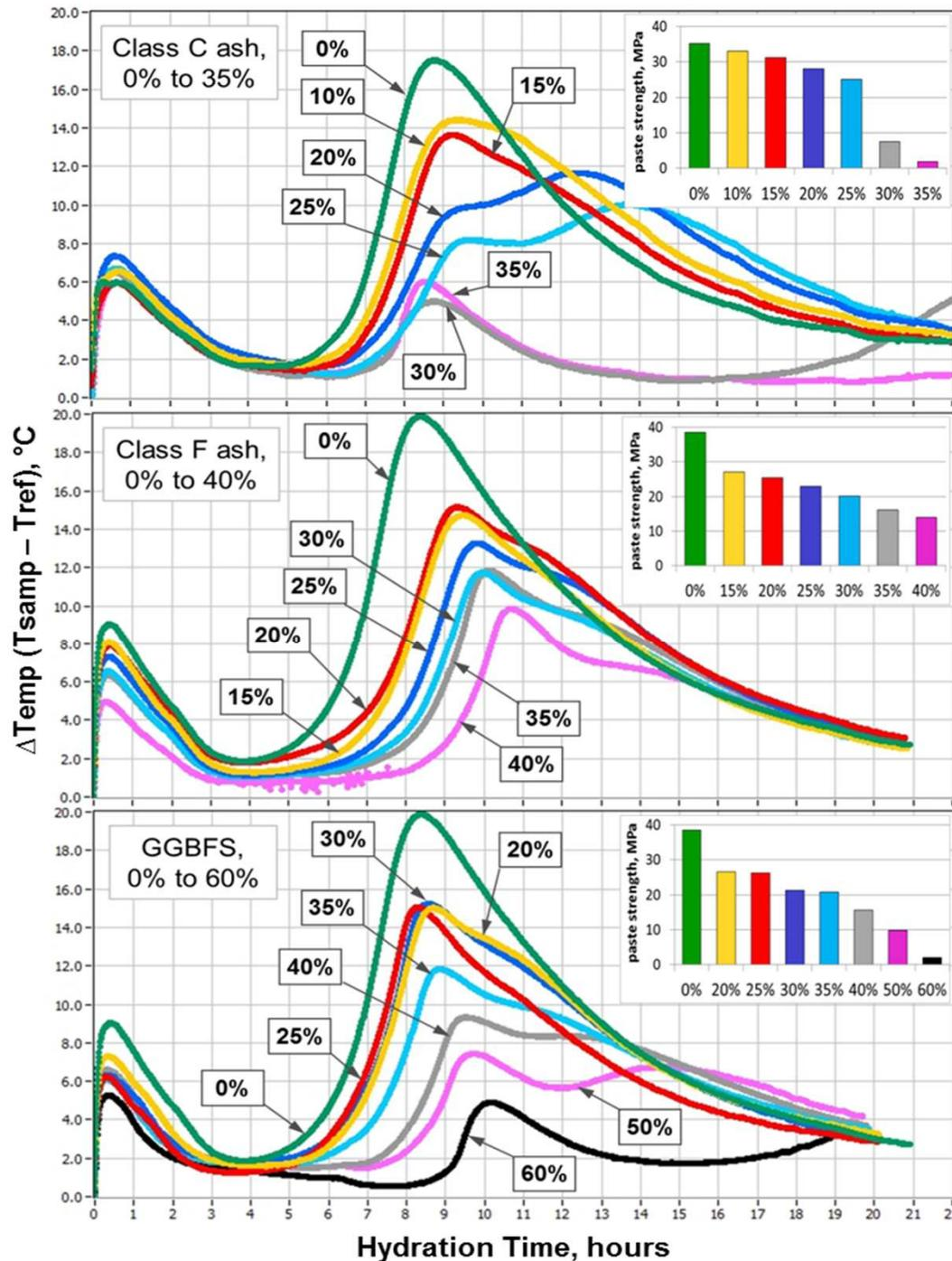
At left, thermal profiles and 1-day strengths comparing 3 SCM's (C ash, F ash, and slag cement) in otherwise identical mixtures, with incremental cement replacement rates. The Type A/D WR admix was selected because of its known high sulfate-demand tendencies.
