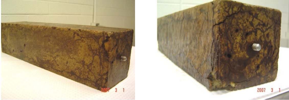
Fig. 6: Condition of concrete prism exposed to the undiluted calcium chloride-based brine for 450 days, and then subjected to 33 freeze-thaw cycles in diluted \text{CaCl}_2 S16p.
