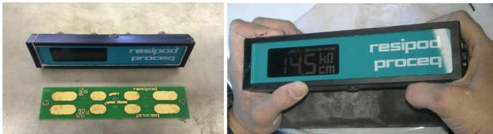
Figure 3- Measurement of Surface Electrical Resistivity by 4-Point Wenner Probe
