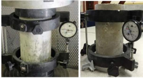
Figure 1 – Measurement of Modulus of Elasticity
