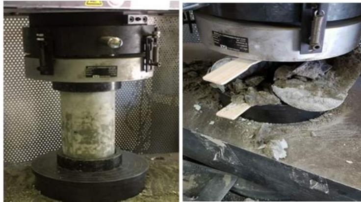
Figure 2- Measurement of Compressive and Tensile Strength
