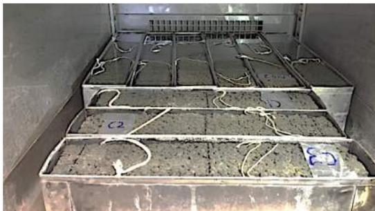
**Fig. 2**—Pervious concrete specimens in freezing-and-thawing chamber (undrained).
