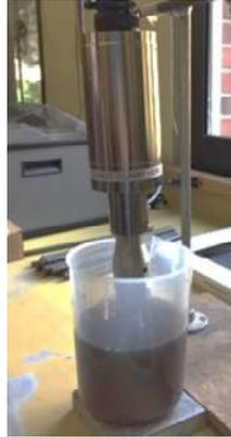
**Fig. 1**—Ultrasonication of GO suspension.
