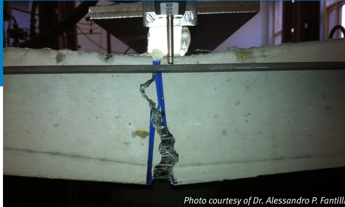
Reduction of Crack Width with Fiber
