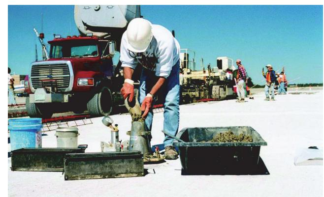
*Fig. 1.3—ACI-certified field technician performing a slump test.*
