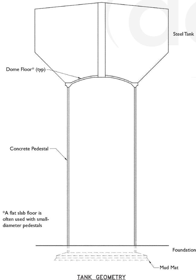
Fig. 1.2b—Common configuration of elevated composite steel-concrete tanks.
