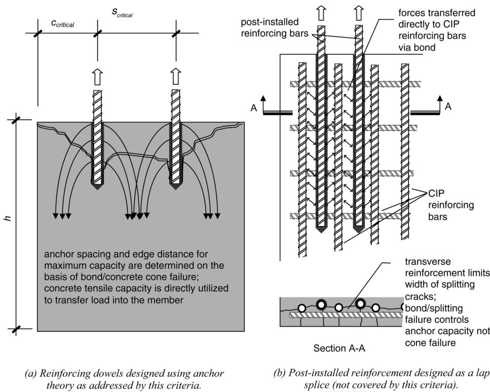
*Fig. R1.1—Examples of post-installed reinforcing bars proportioned with anchor theory and with concepts of reinforcement development and splicing.*
